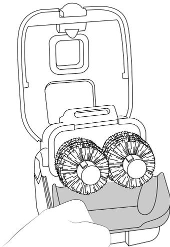
Remove the solder collection tray for disposal of solder waste.
